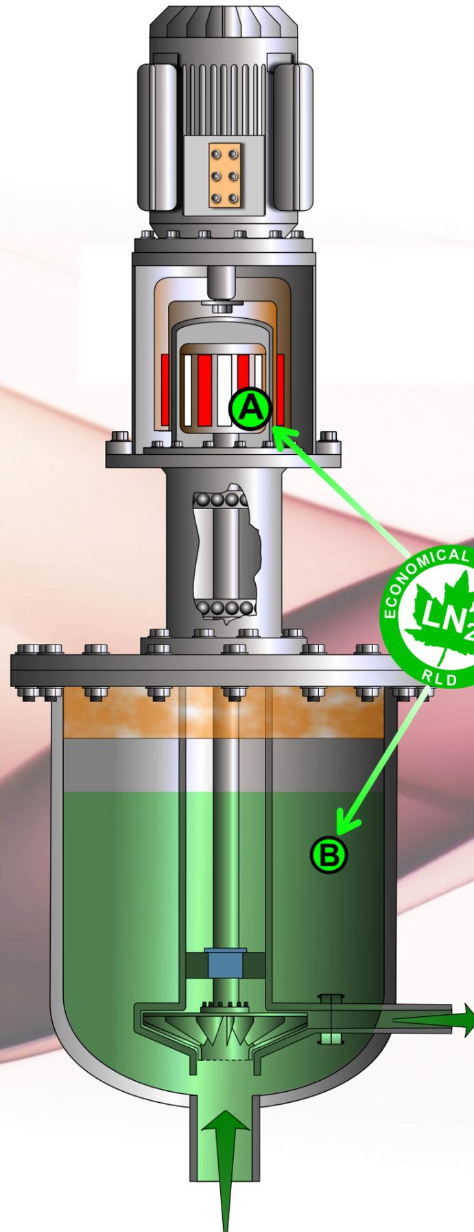
Up till now most pump manufacturers offer hermetically sealed centrifugal pumps for circulation of cold liquids. The range covers canned motor pumps and magnetic drive pumps. Obvious disadvantages of this design are the direct contact of the fluid with the warm mounting casing or flange (C) and the heating of the same fluid by eddy currents (D) generated by the driving motor or magnetic coupling. This heat in-leak results in excessive liquid nitrogen consumption and thus higher operational cost.
