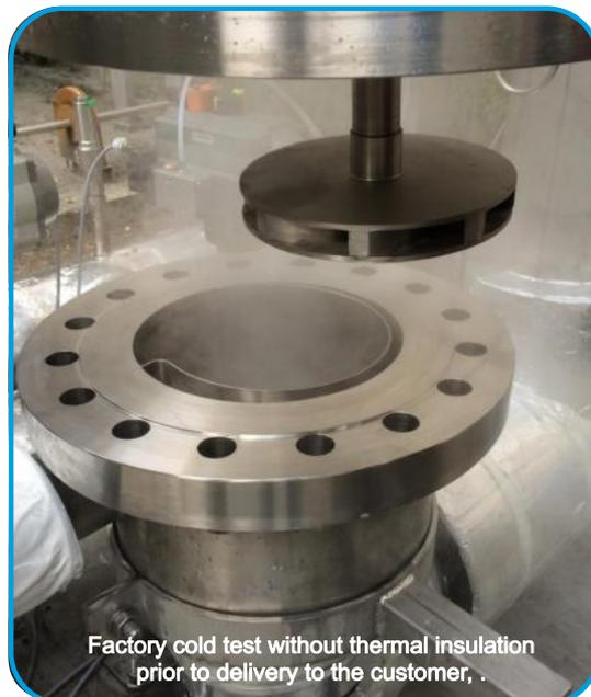
Factory cold test without thermal insulation prior to delivery to the customer.
