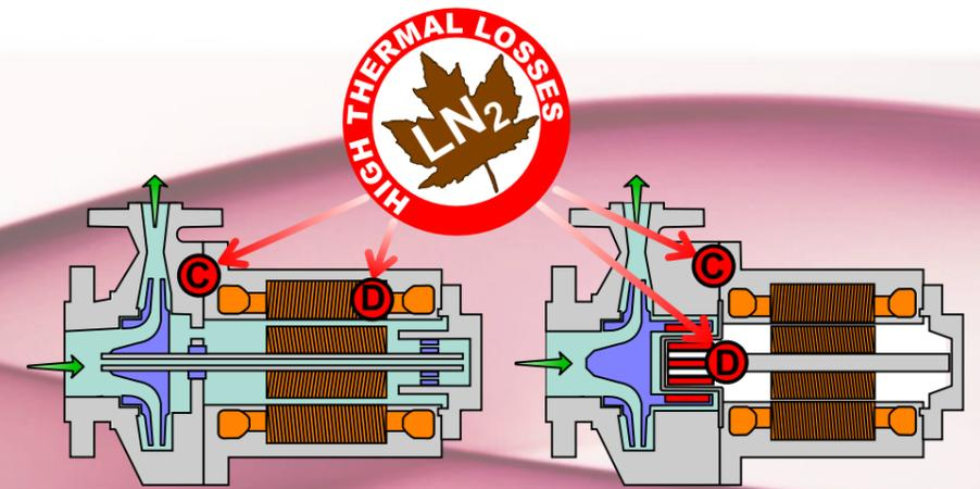
All energy (mechanical or thermal) transmitted to the liquid must be compensated by an equal amount of refrigeration in order to maintain a stable cooling temperature.
