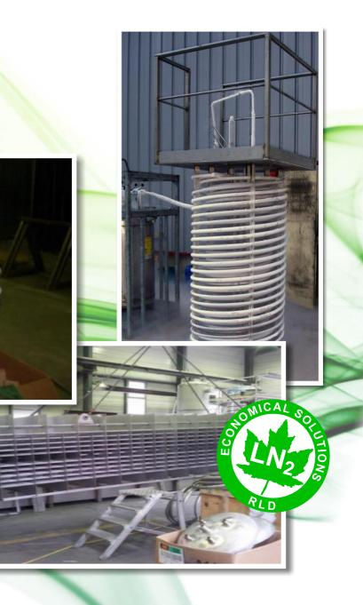
**CRYOWAVE** by RLD is a modular design using tubes optimized with tube inserts for an uniform and improved heat exchange over the total tube length. Moreover, RLD has identified the sub-cooled  $LN_2$  from the storage tank as the origin of flow pulsations.
