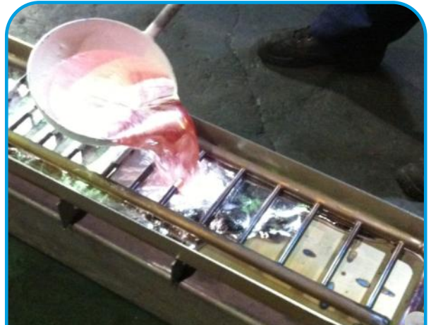
Casting of aluminum for a simple straight heat exchanger
