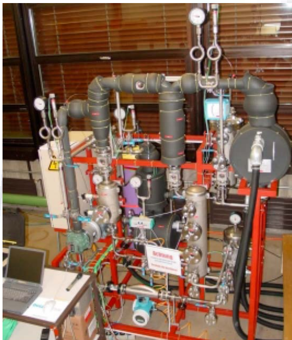
17 kW water-water heat pump prototype (HSR)
