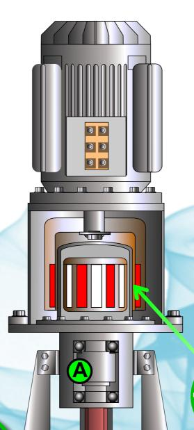
Up till now most pump manufacturers offer hermetically sealed centrifugal pumps for circulation of cryogenic liquids. The range covers canned motor pumps and encapsulated motor pumps. Obvious disadvantages of these designs is the fact that part of the cryogenic liquid is used for the cooling of the drive motor. This results in excessive liquid nitrogen consumption and thus higher operational cost.
