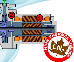
The same remarks are valid for the encapsulated motor version where the fluid is heated by the eddy currents between rotor and
