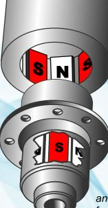
Inner magnets, non-magnetic bell and exterior magnets of a magnetic coupling
